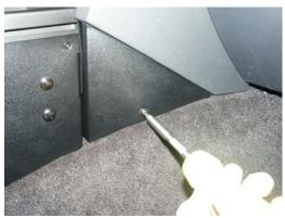
Attach driver and passengerside wire panels (#7 & 8) to frame support bracket using #10 x ½" phillips machine screws and washers.
